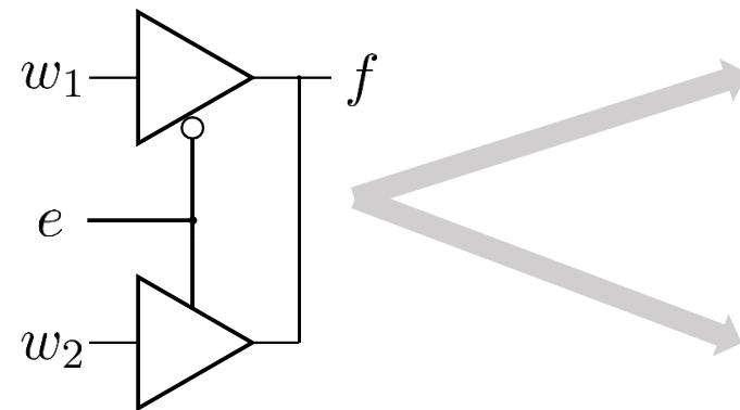
To avoid short circuits, only one driver at a time is enabled
